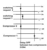
CO05 Delay time at power supply start-up.
