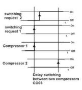
CO04 Off delay time between compressor or stage valve.
